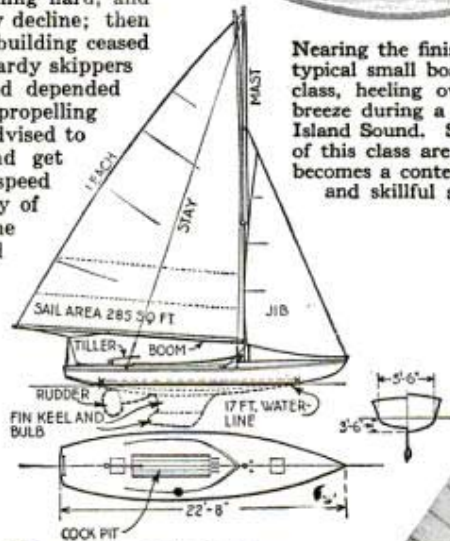
The design and dimensions of the hull and rigging of the Star class boat. Note the jib-headed or leg o' mutton mainsail characteristic of the "Marconi" rigging of boats of this class
