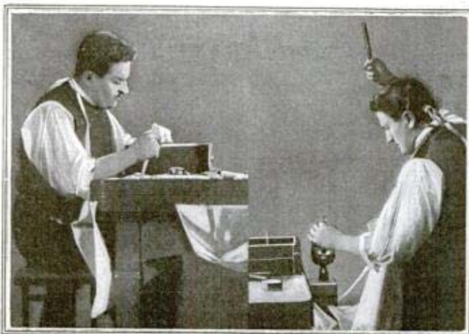
The diamond was a clumsy jewel of dull luster until the art of cutting and polishing it was discovered in the fifteenth century. If the stone is large the first step is to make an incision and then to cleave it with a mallet, which two steps are illustrated by this picture
