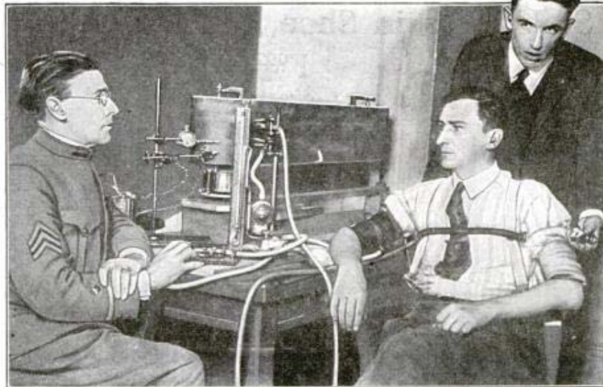
A man can lie, but science has shown that he cannot force his heart and lungs to lie also. A false answer accelerates their action and the apparatus shown above records these variations, revealing the probable falsehood they betray
