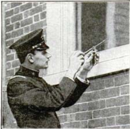
Chemically intensifying fingerprints on a window pane
